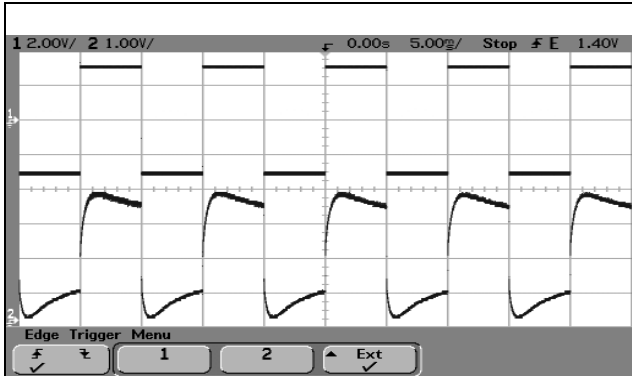
Fig1: up: modulation signal; down: resulting intensity signal. Response at 50 Hz: thermal effect in the impedance matched line translates in phase transients after the sharp edges
