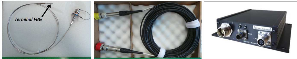
Figure 4 : Complete terminal temperature measurement chain
